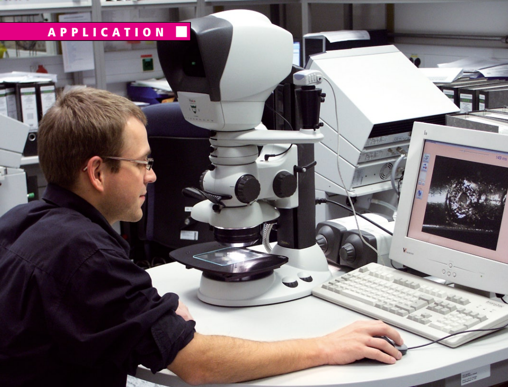
Fig. 1: Inspecting the insulation on a monopolar electrode after a stress test in the ERBE test lab
