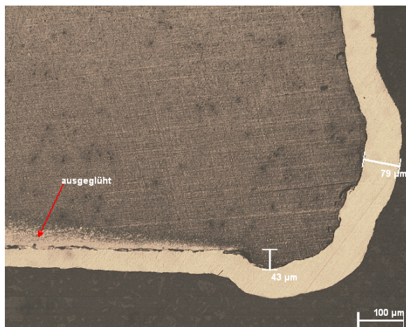
Measuring a chromium/nickel layer with reference to the annealed zone
