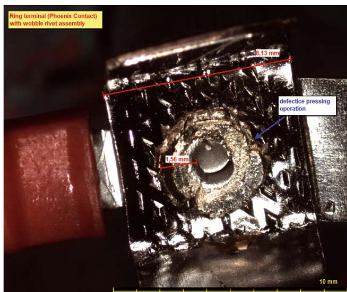
Fig. 3: "Ring terminal" with measurement and label
